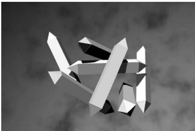
FIGURE 12.4 Gel network of needle-like structures.
