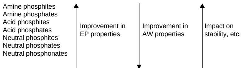
FIGURE 3.23 An approximate ranking of the effect of structure on the AW, EP, and stability properties of the base stock.
