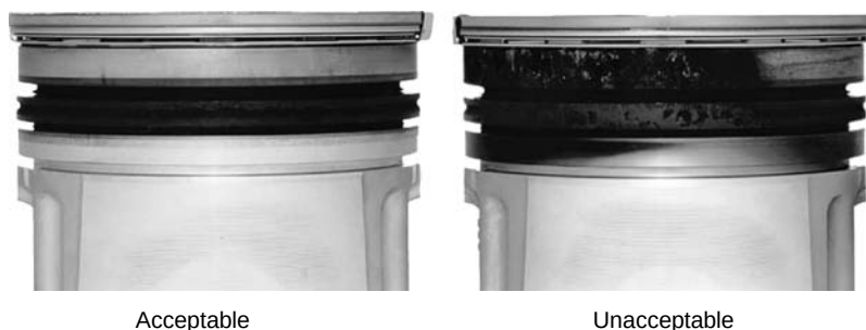
FIGURE 19.6 Detergents keep upper pistons clean.
