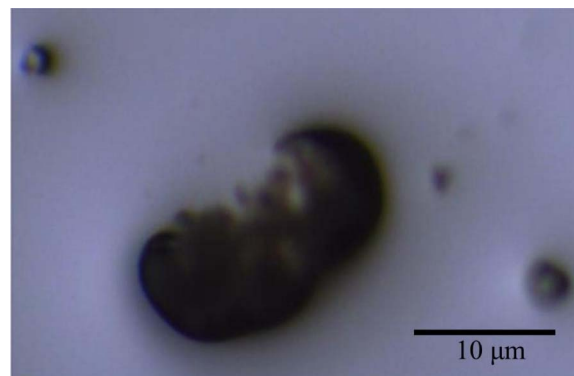
Fig. 5. Part of a microcapsule ruptured at agitation rate above 450 rpm using optical microscopy.
